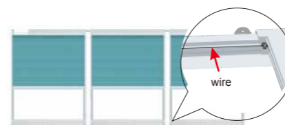
Honey Comb Skylight Track Single Motor (one motor with a few blinds) sketch map
